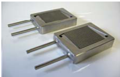
Figure 2a - Commercial 28cm 2 test fixture
