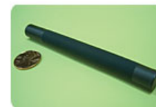
Figure 1. ECOG device with thin-film, Gd-doped ceria membrane.
