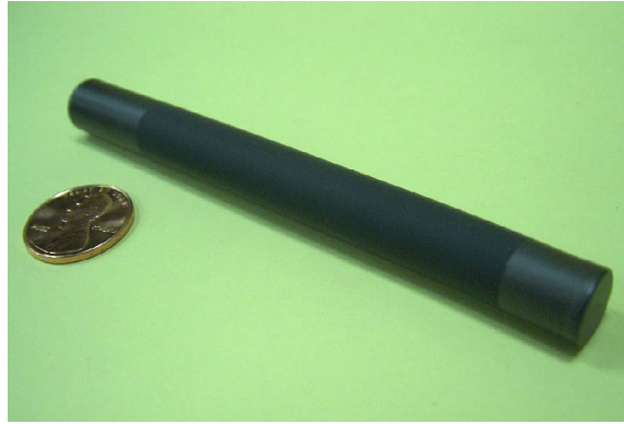
Figure 1 - ECOG Device with Thin-film Gd-doped Ceria Membrane
